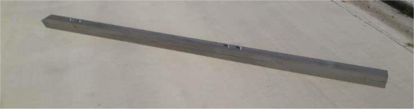
**2** The inside of the post is a galvanized steel tube
